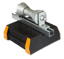
The HBS-MEGA-R Series are designed for superior support of natural gas and refrigeration pipes. The roller allows for longitudinal movements of the pipe. This support is suitable for most types of roofing material or flat surfaces.
